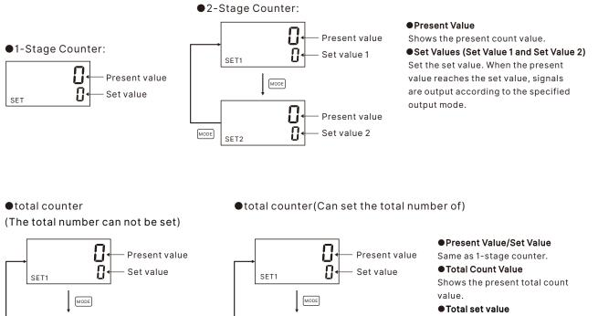
Set the total set value. Total count value When the total value reaches the set Value, total output(OUT1) turns ON.
