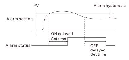
The alarm ON delay also takes effect when the power is turned on. When the interval of the alarm ON is the ON delay setting, the alarm output will not turn ON. Similarly, when the alarm OFF interval is below the OFF delay setting, the alarm output will not be turned OFF.
