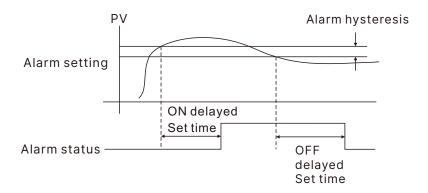
The alarm ON delay also takes effect when the power is turned on. When the interval of the alarm ON is the ON delay setting, the alarm output will not turn ON. Similarly, when the alarm OFF interval is below the OFF delay setting, the alarm output will not be turned OFF.
