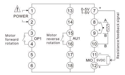
When the valve position feedback signal is a potentiometer, install a non-isolated 5V power distribution output module V5 to convert the resistance signal into a voltage signal (as the picture shows).
