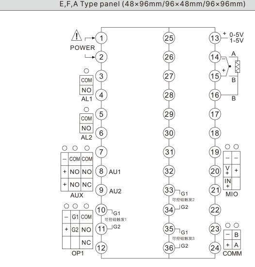
Note: Linear voltage ranges below 1V are input from terminals 14(-) and 15(+), while signals from 0 to 5V and 1 to 5V are input from terminals 13(+) and 14(-); 4-20mA linear current input can be external Connect a 250 ohm high precision resistor to convert it into a 1-5V voltage signal, and input it from terminals 13(+) and 14(-). You can also install I3 and I4 modules on the MIO port to input from terminals 20 and 21.
