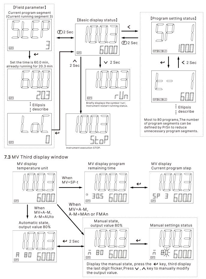
$When \ A-M=FMAn, \ For \ manual \ state \ only \ , \ no \ manual \ / \ automatic \ state \ switch.$
