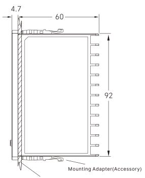
Indicates the cross-section of the cabinet panel. The thickness of the panel must be 1 to 5mm
